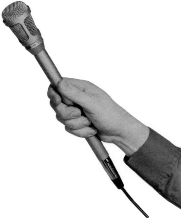
The Model SM82-LC is a hand-held, self-contained, unidirectional, condenser microphone containing its own line level amplifier, peak limiter, and battery. It is designed to provide a line level output for use in a variety of broadcasting situations where a line level microphone with a built-in limiter is required.
