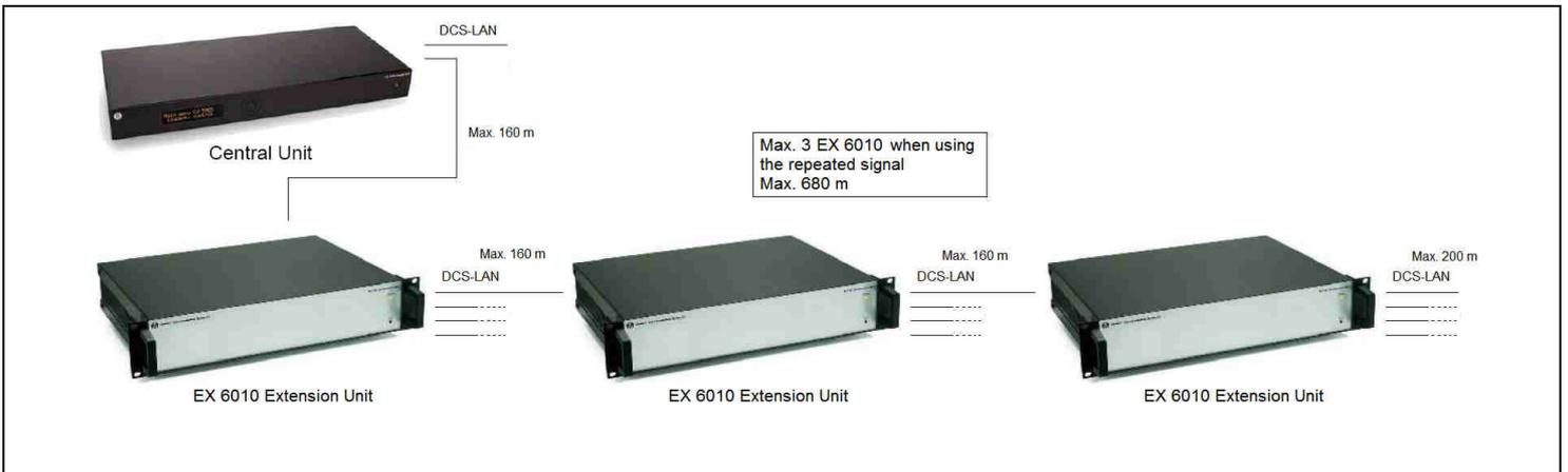
Figure 0-A Repeated Chain connection
