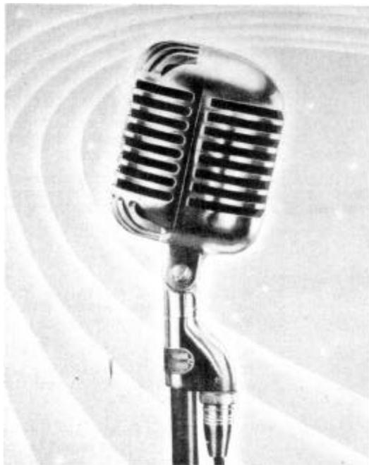
Low impedance models 55A and 55B may be fed into a standard low impedance input amplifier (See Fig. A-3) or into an amplifier with high impedance input (Fig. A-2). In the latter case Shure Model A86A Cable-Type Transformer is available for coupling the low impedance line to the amplifier input. The double-winding primary permits coupling either a 35-50 ohm line or 200-250 ohm line to the high impedance input.
